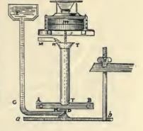
are two apertures in opposite directions. When water from the mill-course m m is introduced into the tube t t. it flows out of apertures a b, and consequently the whole machine is put in motion by the reaction of the water. The bridge tree is elevated or depressed by turning the nut at the end of the lever.
