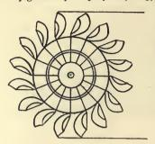
form, so as to be concave towards the stream; and notwithstanding certain defects, these wheels are always superior to those with flat floats, since, in the former case, the water acts by its weight as well as by its impact. [Curved floats, it will be remembered, are found in the ancient Irish specimen already illustrated.]
