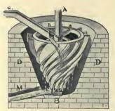
vertical axis in the chamber to D, in the diagram annexed, and is driven both by the impulse of the water from CC and, when the impulse is spent, by the weight of water as it descends along the spirals.
